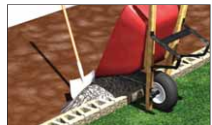
Backfill behind and in blocks, level and compact. Sweep top of blocks.
