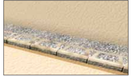
Backfill wall rock and infill soils.
